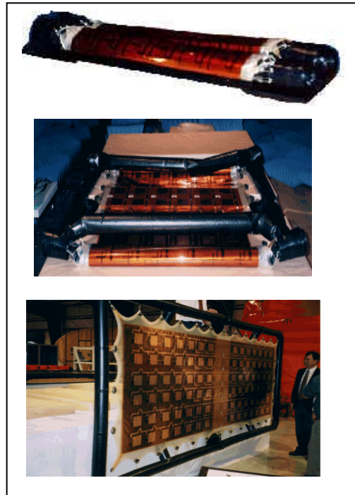
Fig. 1. JPL's 1x3m passive membrane antenna. The top figure shows the antenna in stowed configuration. The antenna is partially deployed in the middle figure. The fully deployed antenna is shown in the bottom.
